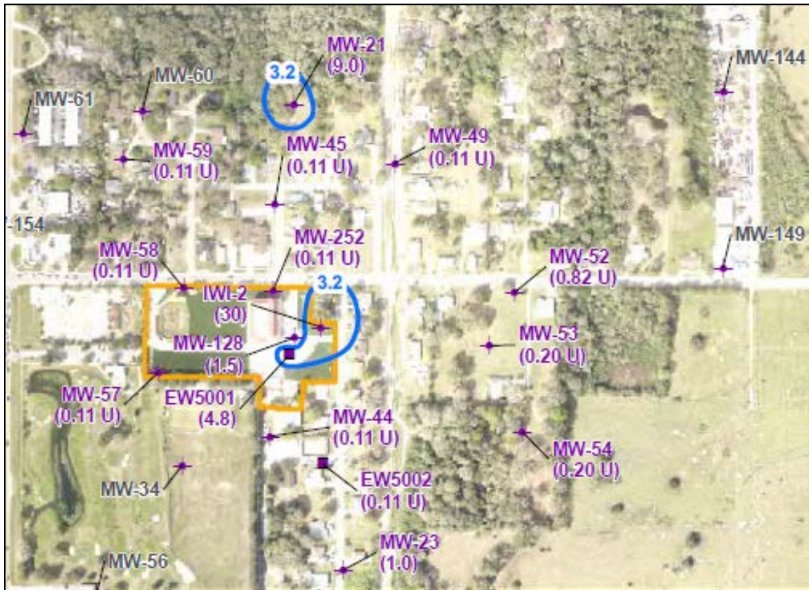
Figure 6 – 1,4-Dioxane Concentrations in the Salt & Pepper Sands (from Figure 15A of the 2020 RASR)
